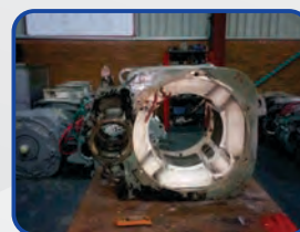
Completed Traction Motor Stator Awaiting Armature for Final Assembly
