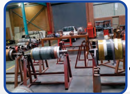
Armature Rewinding Section
