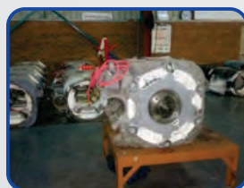
Completed Traction Motor
